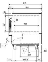
Drain Electrical inlet (power)
